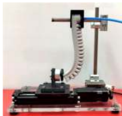
Fig. 3 Force measurement by adaptive push button switch machine.
