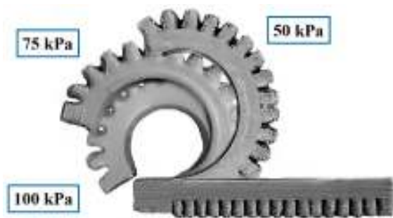
Fig. 6 Soft actuator movements in several air pressure among 50 kPa to 100 kPa.
