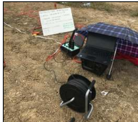
Fig. 7 Equipment used for the Seismic Refraction test
